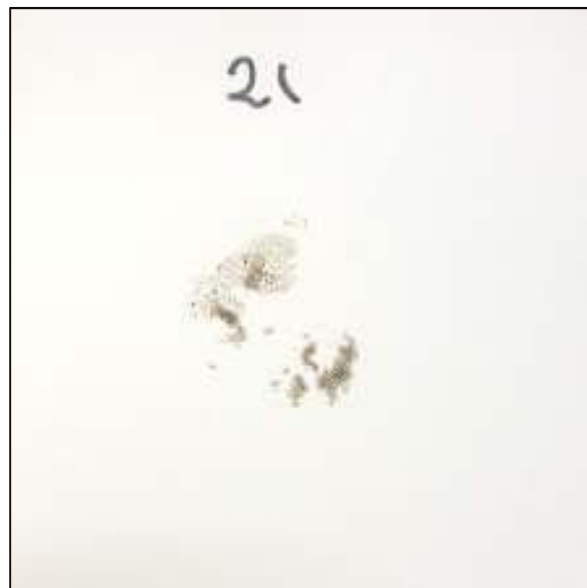
Chemical Spot Test 21, Furfural, Rating 2, Staining
