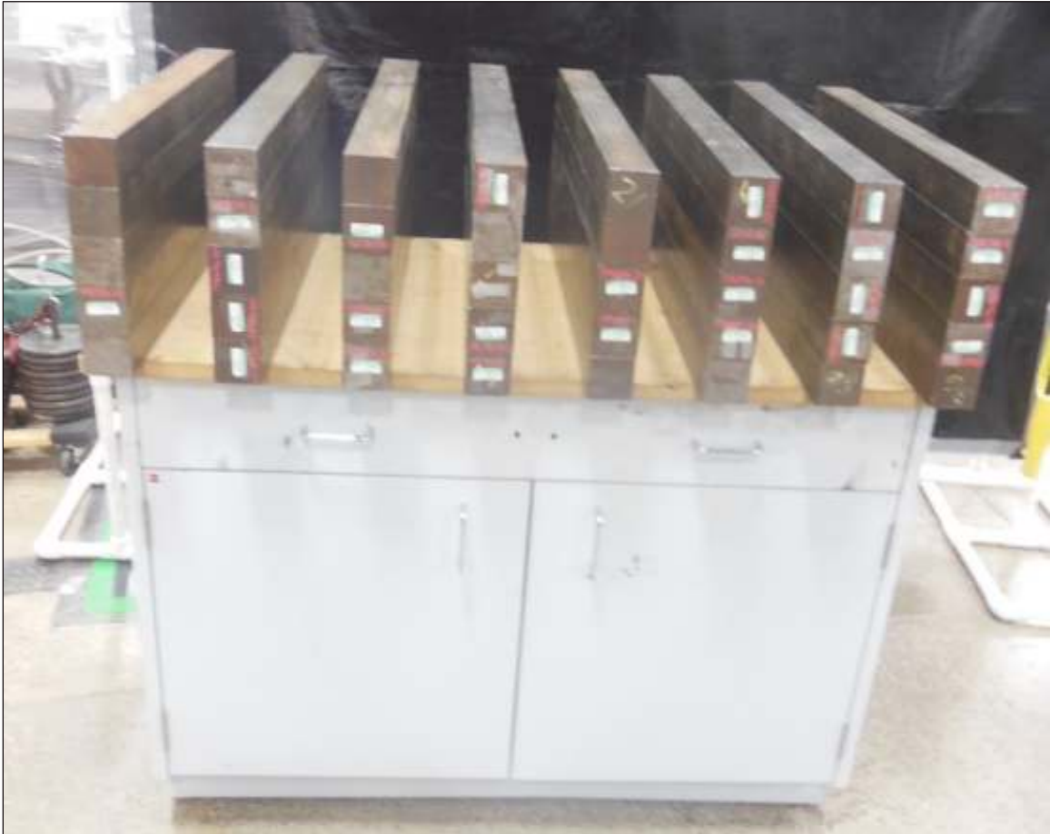
Cabinet Load Test
