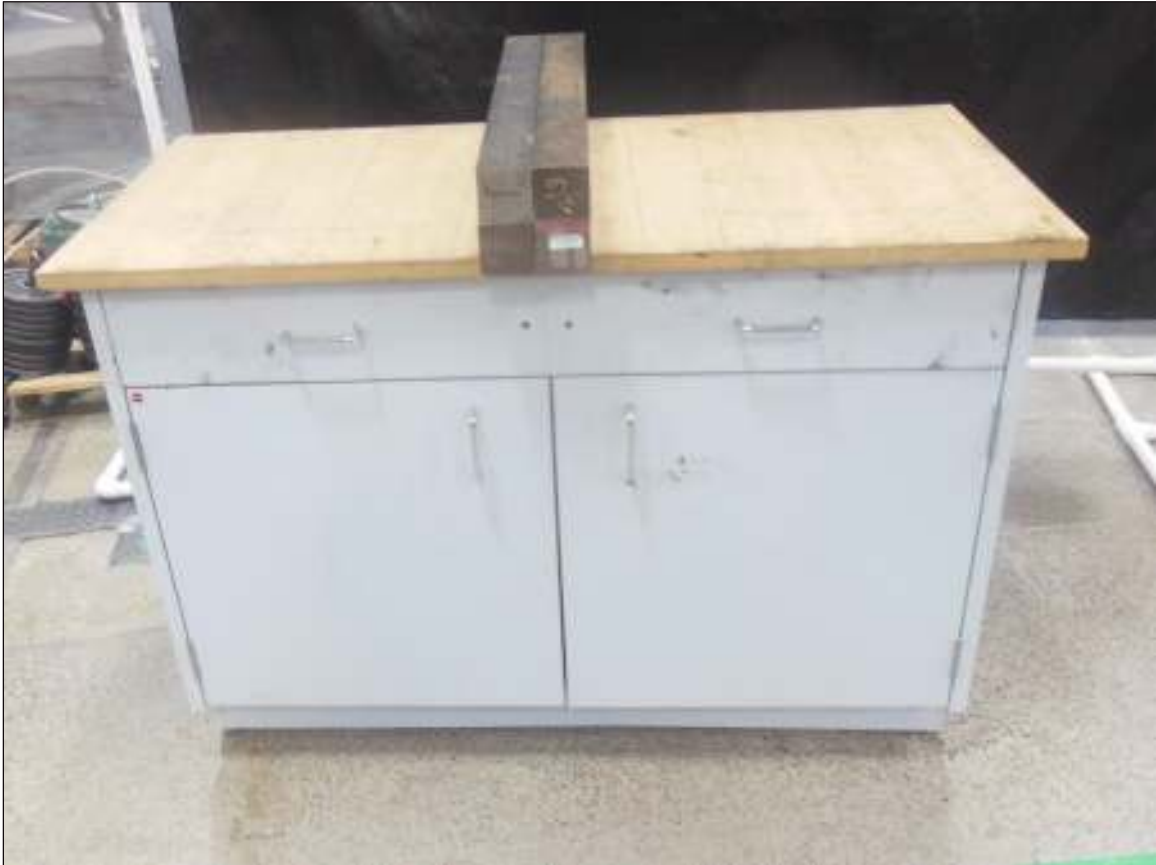
Cabinet Concentrated Load Test
