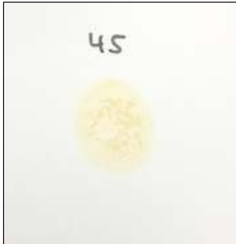
Chemical Spot Test 45, Sulfuric Acid (77%) and Nitric Acid (70%) equal parts Rating 3, Surface Erosion
